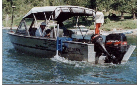
Skagit River Instream Flow Measurements Using the ADCP
